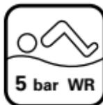
If "WATER RESISTANT 5 BAR" is inscribed on the case back, your watch is designed and manufactured to withstand up to 5 bar and is suitable for swimming, yachting and taking a shower.
