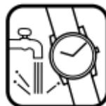
If "WATER RESISTANT" is inscribed on the case back, your watch is designed and manufactured to withstand up to 3 bar, such as accidental contact with splashes of water or rain, but it is not designed for swimming or diving.
